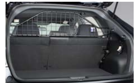
48 Dog guard (K/M) F555EFG000 W Separates cargo room from passenger area, applicable for ISOFIX childseat.
