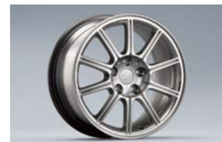
27 Alloy wheel 10-spoke, Platinum silver (17 inch) 28111FE371 W 8"x17" offset 53 PCD 114,3 Tyre size 235/45R17
