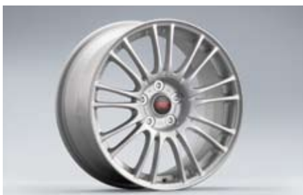
20 Alloy wheel 9-spoke, Silver (18 inch) 28111FG070 W 8.5"x18" offset 55 PCD 114,3 Tyre size 245/40R18
