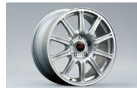
23 Alloy wheel 10-spoke, Silver (17 inch ) 28111FE272 W 8"x17" offset 53 PCD 114,3 Tyre size 235/45R17
