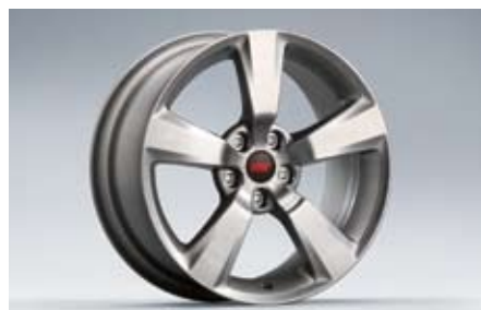
21 Alloy wheel 5-spoke, Lusteric silver (18 inch) 28111FG050 W 8.5"x18" offset 55 PCD 114,3 Tyre size 245/40R18
