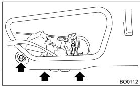
4) Disconnect connectors, and then remove rear gate latch assembly.
