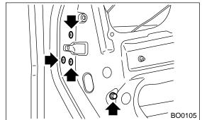
5) Disconnect the connector. Remove the front door latch assembly.
