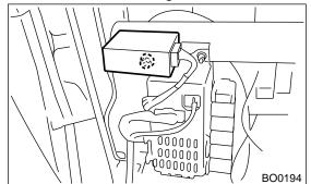
4) Disconnect keyless entry control module and the other electrical control module.
