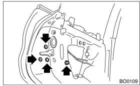
5) Disconnect the connector, and then remove the rear door latch assembly.
