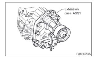
2) Remove transfer driven gear and center differential as a set.
