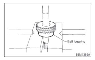
2) Install ball bearing to transfer driven gear.
