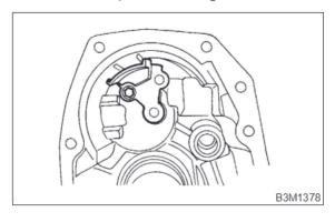
2) Install reverse check sleeve assembly to transfer case.
