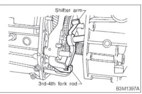
3) Install transfer case with extension assembly to transmission case.
