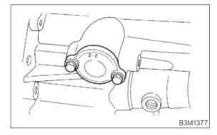
3) Install ball, reverse accent spring, washer and plug to transfer case.
