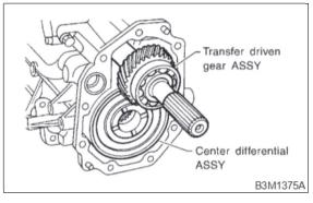
2) Measure height "W" between transfer case and ball bearing on the transfer driven gear.
