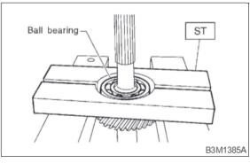
2) Using ST, remove ball bearing from transfer driven gear.
