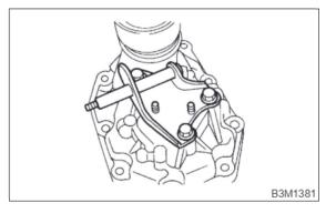
3) Using ST, remove ball bearing from transfer drive gear.
