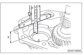
4) Calculate space "Y" using the following equation: Y = X - W + 0.24 mm (0.0094 in) [Thickness of gasket]
